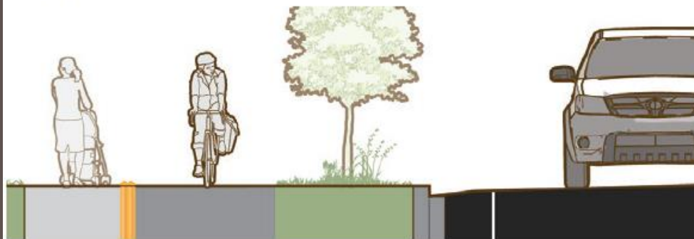
Figure 4-19. Separated bike lanes may be configured on an existing roadway surface by using a physical barrier such as a curb or median to separate the bikeway from the roadway.
